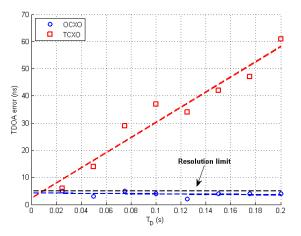
Fig. 1. TDOA error as a function of  $T_D$  for two different types of oscillators. For an OCXO, the TDOA error is below the resolution accuracy, but for the TCXO the effect of clock skew can clearly be seen.
