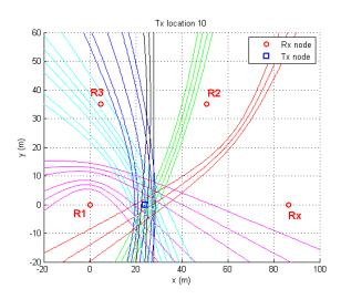
Fig. 3. Hyperboles corresponding to the TDOAs measured with three relay nodes and one receiver. The blue lines correspond to the TDOA between Rx and R1, the red lines between RX and R2, the green lines between Rx and R3, the cyan lines between R1 and R2, the magenta lines between R1 and R3, and the black lines between R2 and R3.
