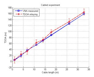
Fig. 2. Measured TDOA for a cabled setup with different cable lengths. The real TDOA, measured with a VNA, is shown for reference.
